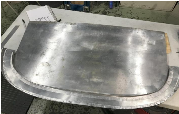
The new wall of the lower turret with the rib
