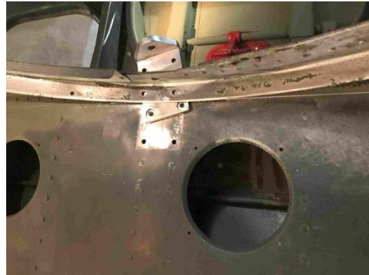
Metal bracket cleaned and ready to reattach
